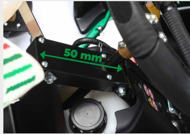
The cushioned steering column, with its guaranteed 5 cm controlled movement, allows energy to be dissipated in the event of a collision, thereby safeguarding the driver's upper limbs.
