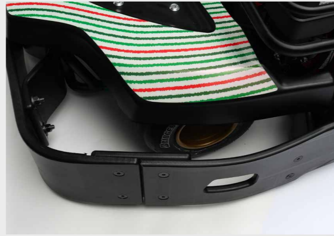
At the rear, any collisions are cushioned by the perimeter fairing that it is mounted on polizene supports with a deformable structure and a specific shape made to absorb shocks.
