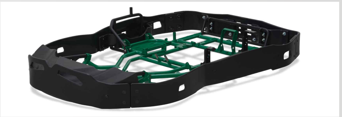
At the front, there is a polyurethane shock absorber, positioned inside the fairing and covered by a removable cover. This shock absorption system has been combined with a protective perimeter band, made from black polizene, which also absorbs shocks and allows the kart to slide along the barriers in case of collision, thereby safeguarding the driver.
